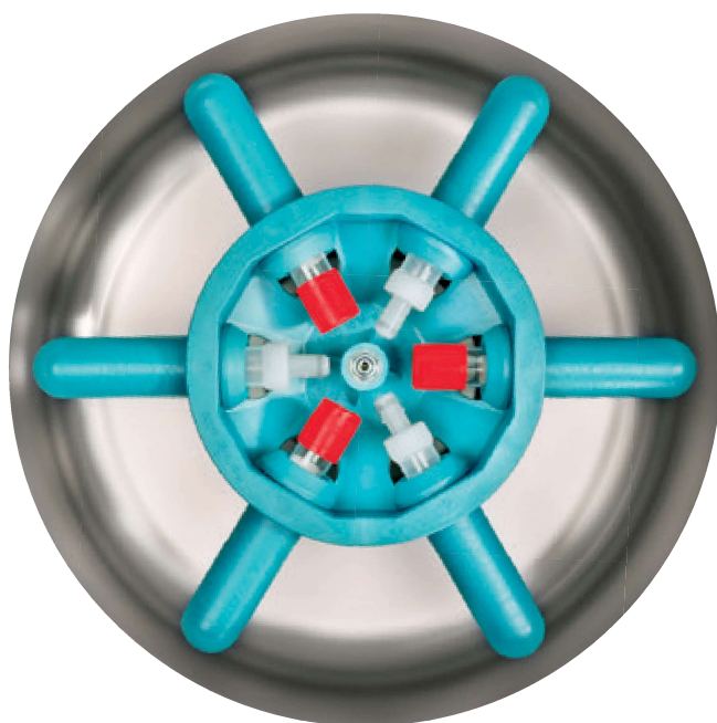
View into the centrifuging chamber showing the rotor with carriers and blood collection tubes swung out by 90 degrees.
